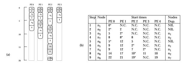
Figure 7: (a) The schedule generated by the CPFD algorithm (schedule length = 20); (b) the scheduling steps of the CPFD algorithm (a node is scheduled to the processor on which the start time is marked by an asterisk; an entry with "N.C." indicates the processor is not considered).
